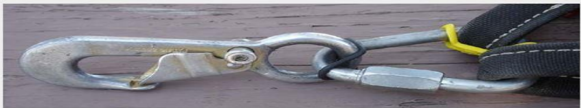
— "J" hook, Tri-link, and an "O" Ring, correctly installed. USFS photo.
