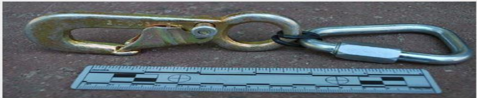
— "J" hook, Tri-link, and an "O" Ring, incorrectly installed. USFS photo.
